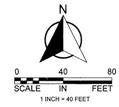
BASIS OF BEARING SYSTEM ALL BEARINGS ARE IN RELATIONSHIP WITH THE WEST LINE OF OUTLOT D, PIONEER COMMONS WHICH IS ASSUMED TO BE N00°56'17"W
