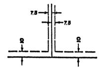
BEING 75 FEET IN WIDTH AND ADJOINING SIDE LOT LINES, UNLESS OTHERWISE INDICATED, AND BEING 10 FEET IN WIDTH AND ADJOINING STREET LINES AND REAR LOT LINES, UNLESS OTHERWISE INDICATED ON THE PLAT.
