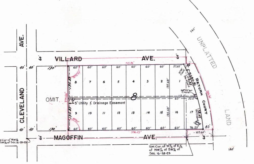
Thereby certify to having surveyed the property described on this plat as Murray-Lane Addition Plat-3 and have placed iron monuments at the corners as shown and the same is correct. There is no low wet ground nor any traveled road or easement on or across same except as shown.
