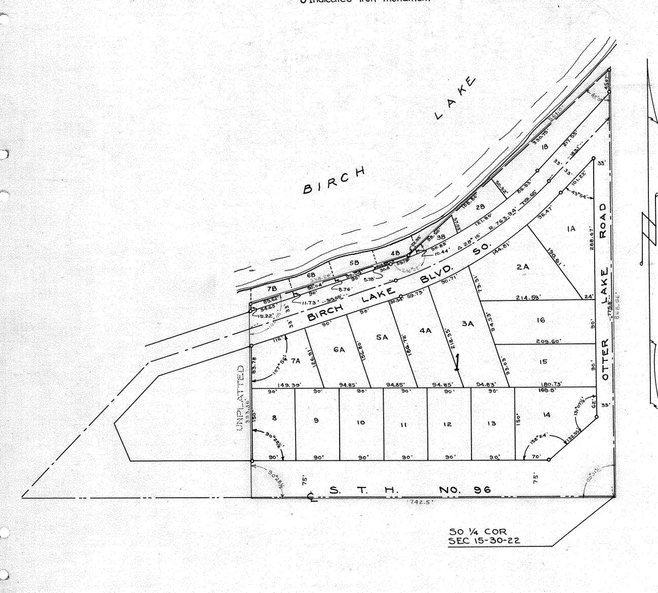
I hereby certify to having surveyed the property described on this plat as Brennan Addition and have placed iron monuments at the corners as shown and the same is correct. There is no low wet ground nor any travelled road or easement on or across same except as shown.
