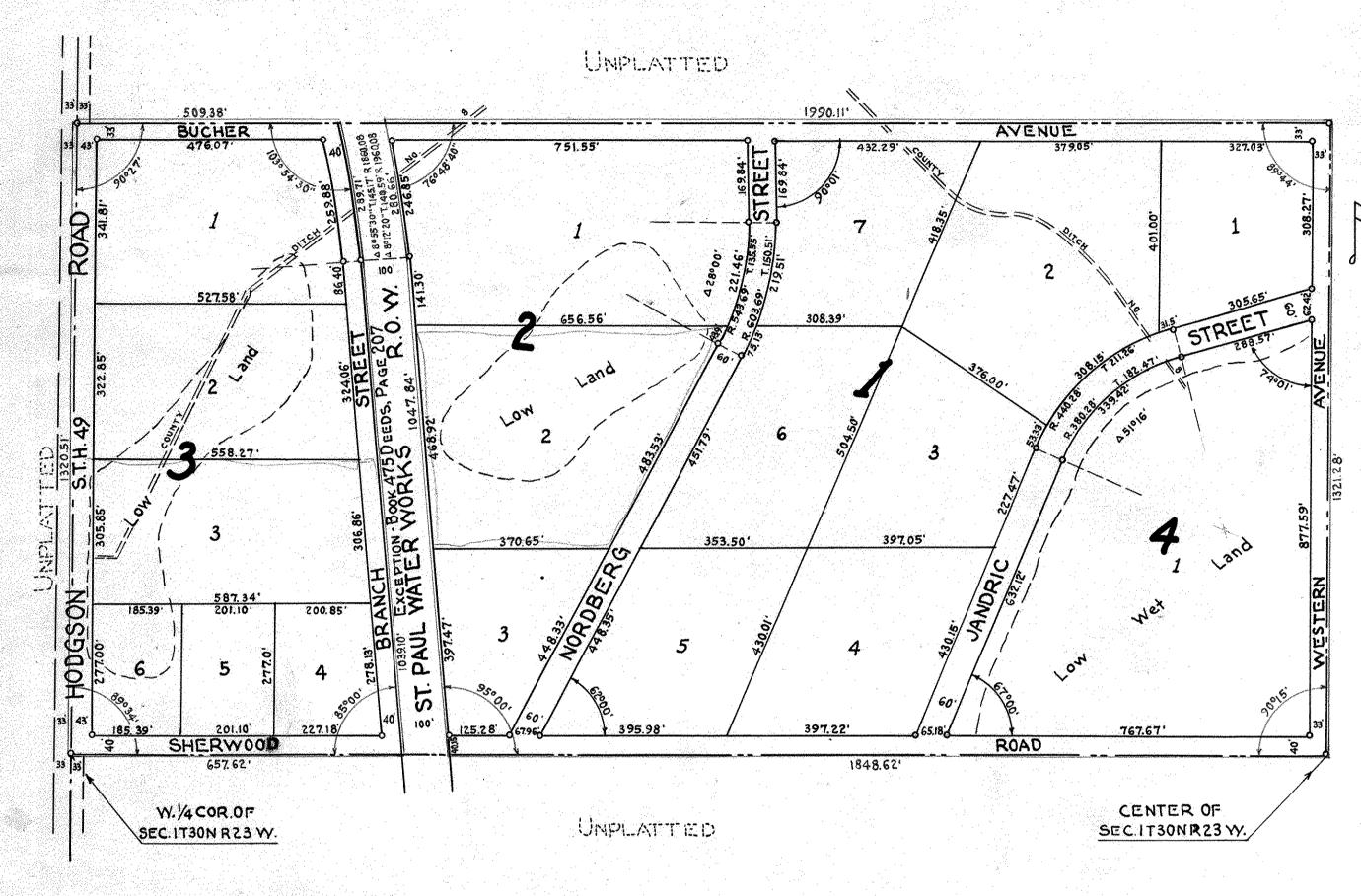
I hereby certify to having surveyed the property described on this platas \*BUCHER ADDITION \* and have placed irons at the corners as shown and the same is correct. There is no low wet ground nor any traveled road or easement on or across same except as shown.
