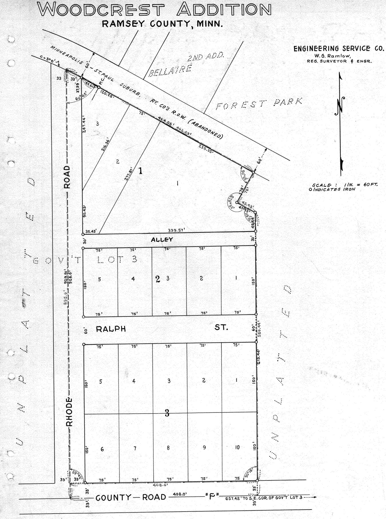
I hereby certify to having surveyed the property described on this plat as "Woodcrest Addition" and have placed irons at the corners as shown and the same is correct. There is no low wet ground nor any traveled road or easement on or across same except as shown.
