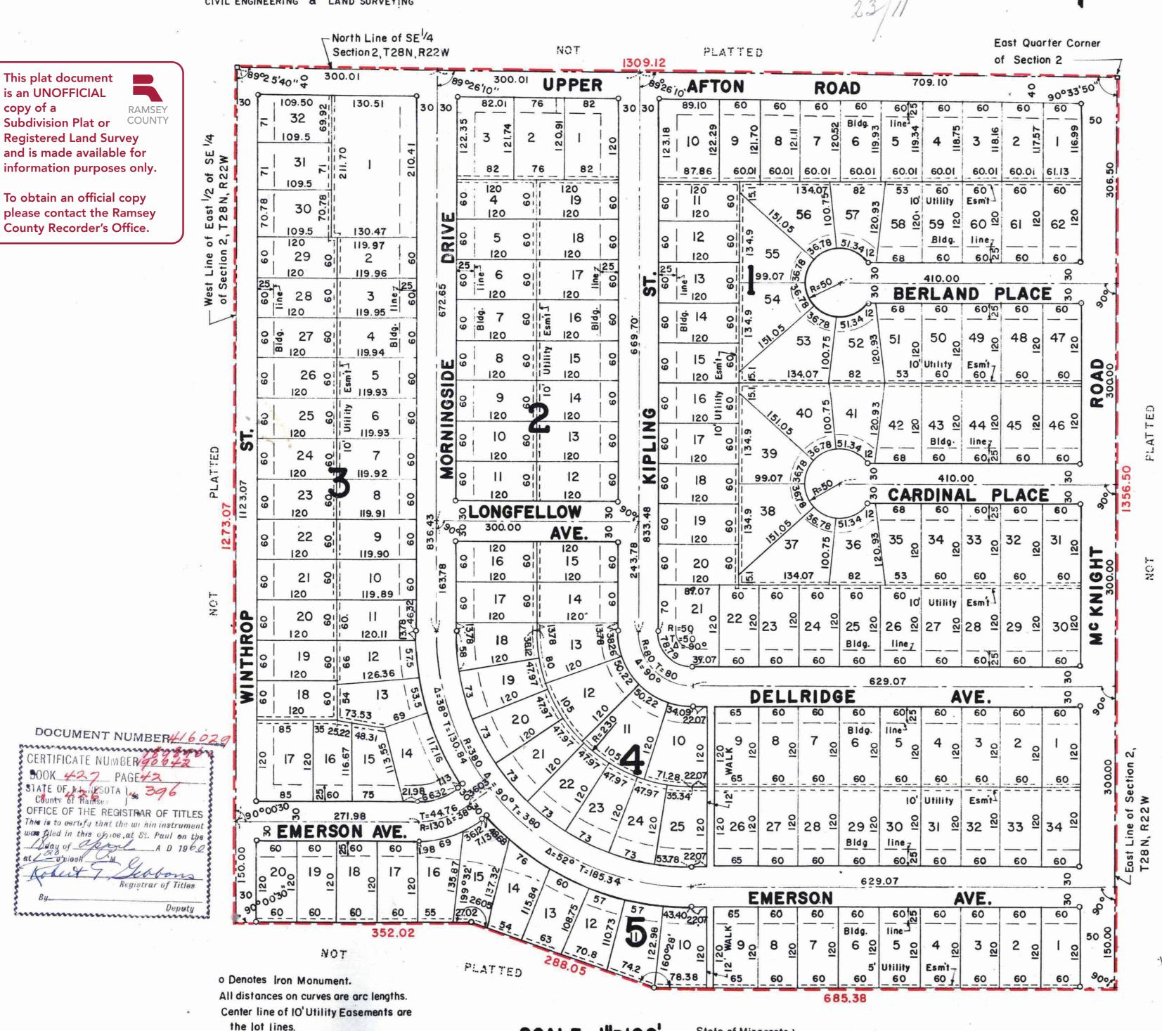
I hereby certify to having surveyed the property described on this plat as Afton Heights Addition and have placed Iron monuments on the corners shown and the same is correct. There is no low wet ground nor any traveled road or easement on or across same except as shown.
