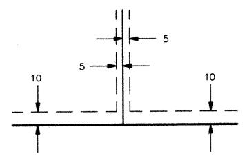
BEING 5 FEET IN WIDTH AND ADJOINING LOT LINES, AND 10 FEET IN WIDTH AND ADJOINING STREET LINES AND REAR LOT LINES, UNLESS OTHERWISE INDICATED ON THIS PLAT.
