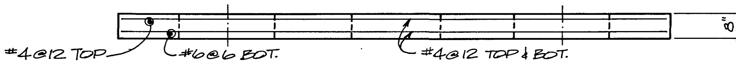
SECTION - COVER SLAB
