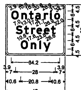
WZ-10; 3.0" Radius, 1.0" Border, Black on Orange; [Ontario] E Mod; [Street] E Mod; [Only] E Mod;
