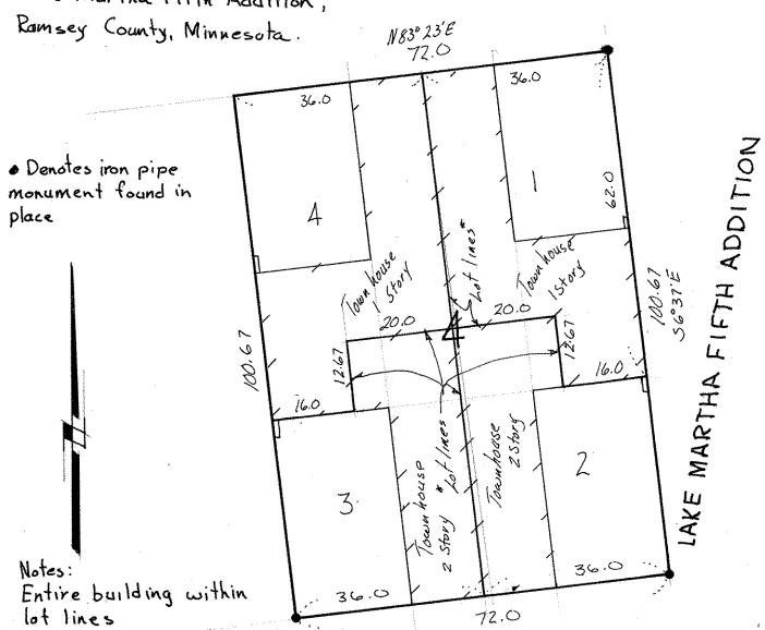
\*Lot lines Denotes where Center line of Fnd wall is on lot line and above Fnd there are two 4" walls Seperated by an air Space
