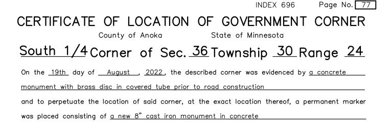
AND on the <u>30th</u> day of <u>September</u>, <u>2024</u>, said permanent marker was <u>reset flush using</u> <u>historical ties</u>. Verified position by RTK GPS method. Updated ties.
