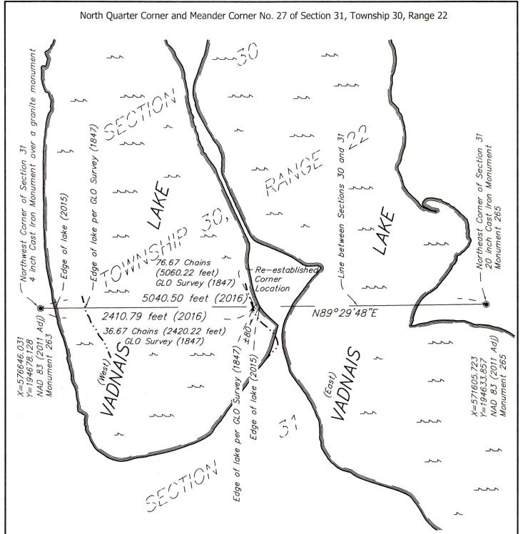
The position of the North Quarter Corner and Meander Corner No. 27 of Section 31, Township 30, Range 22 was established by single line proration between the Northeast and Northwest Corner for said Section using GLO distances and modern measurements taken between the same two corners.
